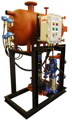
The Arbe ACR-CT & AT condensate recovery packages offer fully certified recovery solution for the collection of condensate from various systems. The unit is a standalone unit and is designed to operate within the requirements of the application. The tank, pumps and pipework are all manufactured from various materials such as carbon steel or stainless steel. The receivers are designed and manufactured in accordance with PD5500 and are fully certified by our 3rd Party Insurance partners.
