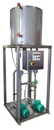
The Arbe range of ACR-N condensate recovery packages offer a reducedfootprint, compact solution for the collection of condensate from various systems. The unit has been designed to offer a solution where floor space is critical, so the condensate tank is located over the pumps and controls.
